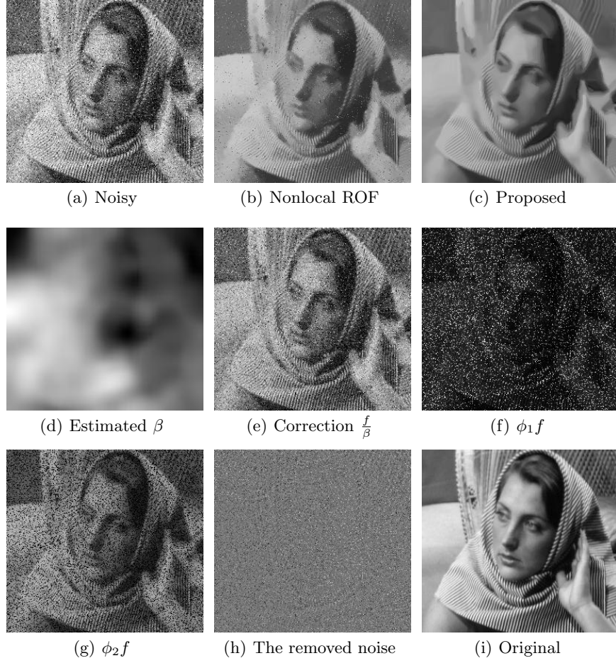
Fig. 1. A Comparison of nonlocal ROF [7] and the proposed model. (a)noisy image with PSNR= 17.01; (b) result with nonlocal ROF, PSNR= 23.94; (c) u , result with the proposed model, PSNR= 27.34 ; (d) the estimated bias function \beta ; (e) the corrected image \frac{f}{\beta} ; (f),(g) the estimated pixels with high level noise and low level noise, respectively; (h) the removed noise by the proposed method, i.e. \frac{f}{\beta} - u ; (i) the original image.
