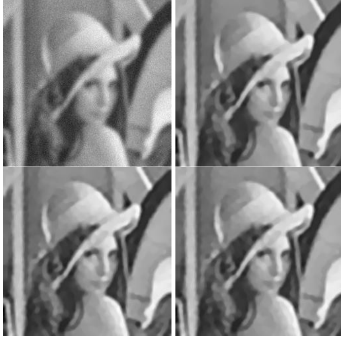
Figure 5: Top left: the blurred image with uniform Gaussian noise; top right: the result of the ROF model; bottom left: the result of the G-TV model; bottom right: the result of the GM-TV model
