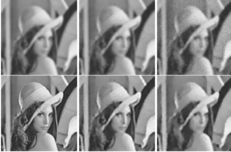
Figure 4: Top: the blurred images with different levels of noise; bottom: restored by the G-TV model.
